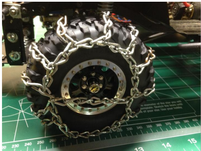
Homemade snow chains for added traction in the snow.
