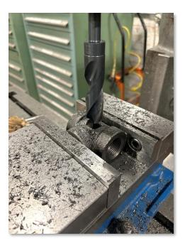
Combustion chamber – Modifying a cast iron "T" fitting that will be the combustion chamber.
