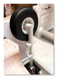
Simulated OLEO suspension is just one of the many scale features on the T-28
