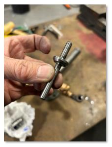
Exhaust valve after silver soldering and machining
