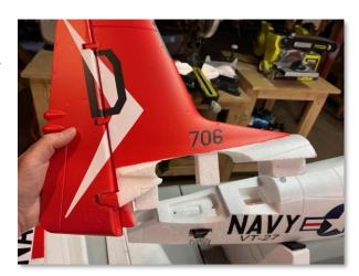
The vertical stabilizer must be removed in order to attach the horizontal stabilizer. The instructions are not clear on this step
