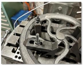
Flywheel mounted to the lathe for drilling and balancing
