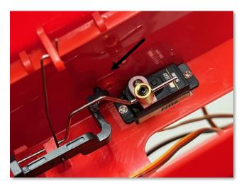
The pin that holds the nose gear mechanism in place had popped out during shipping. It was an easy fix but a good lesson to check over all parts of a plane before flying.
