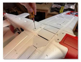
Only four screws and two plastic brackets hold the wings onto the fuselage. Two wing spars held to add rigidity to the wings
