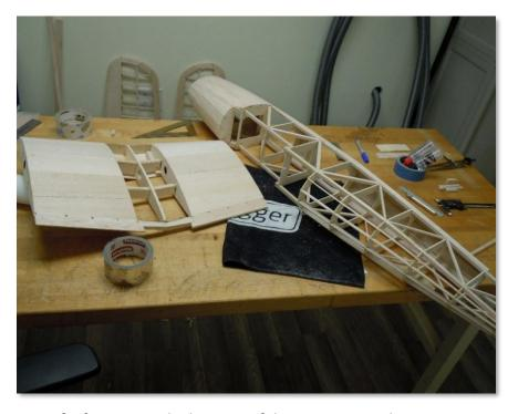
The plans, however, provided a key piece of information: the location of the wing root with respect to the fuselage. The wing center section mounts to the fuselage with 4 wood screws and can be removed if necessary. During normal operation it remains attached to the fuse.
