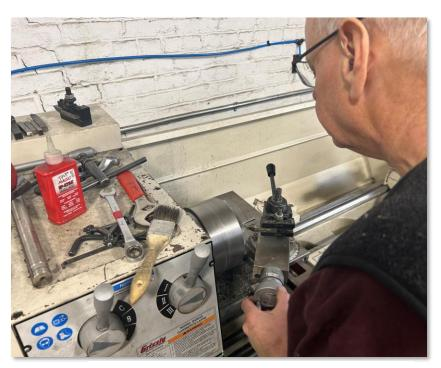
Machining the exhaust valve using the lathe
