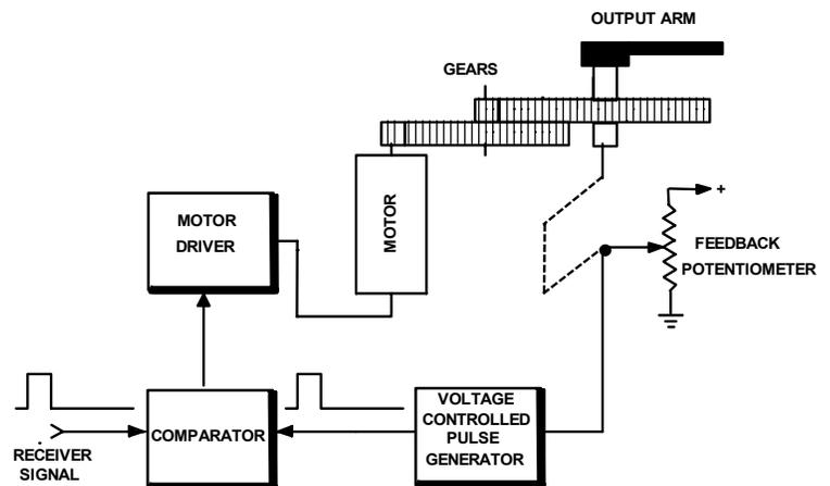
digital function. Measurement of the input signal's pulse width, compared with the potentiometer voltage value determines the motor control signal polarity.
