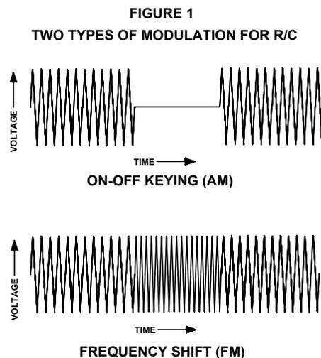
What is correctly stated in these terms is the “P” for pulse. All control information is sent in the form of either discrete on-off of the RF amplitude in the case of AM or a step shift of frequency in the case of FM.
